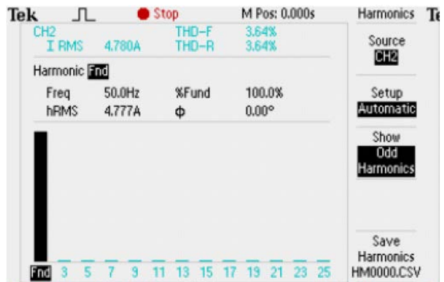
Figure 14. Measured frequency spectrum of inverter output current
